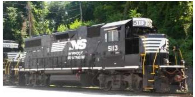
Here is a new comer to the NS yard in Richmond. On July 1st I photographed NS 5113 waiting for its next call to duty. The unit is a rebuilt gp38-2 with a new admiral cab from Juniata Shops in May 2015. The unit was converted from a former Southern Rwy hi nose long hood forward unit.
